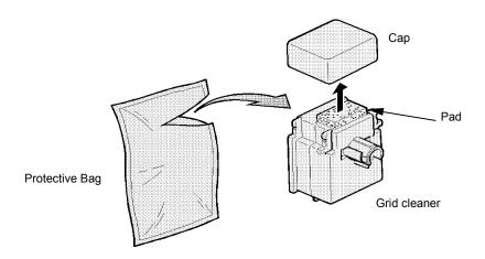
2. Attach the grid cleaner to the printer with the pad facing up as shown in the figure.
